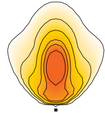
E-GL4F03C2 fixture mounted at 20 feet with 60° tilt.
