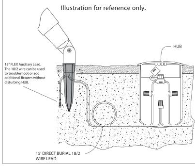
Fasten the fixture to the stake by threading the 1/2" threads into the 1/2" insert. While holding the fixture stationary rotate the stake clockwise until snug. Do not overtighten. Allow the wire leads to rotate freely while fastening the fixture.
