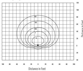
**Note:** All published photometric testing performed to IES LM-79-08 standards. Fixture photometry was completed on a single representative fixture. Foot candle levels are noted inside graph. **Visit e-conolight.com for the latest EPA data**.
